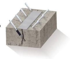
b. To fill cracks with polyurethane, should grout again before the material become solid.
