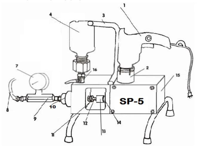
1. Electric Drill 2. Electric Drill Fix 3.Lifting Handle 4. Inlet Tub 7. High Pressure Gauge
